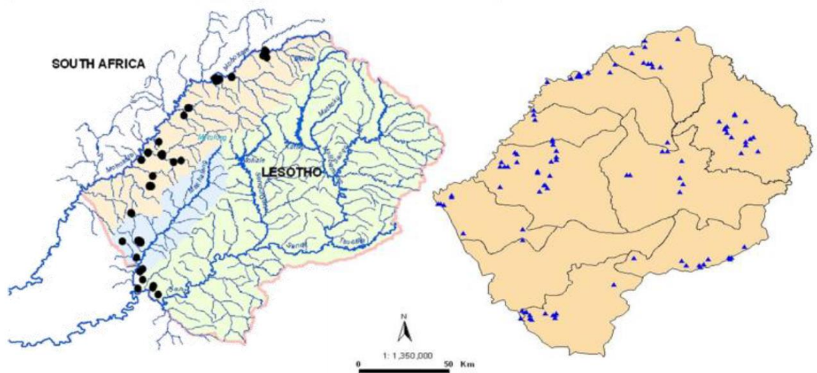
Figure 3-2 Location of monitoring boreholes (left) and springs (right)
