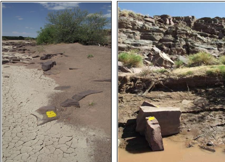
*Figure 8. Examples of strand lines marked on 16 February 2012 and corresponding to a peak discharge of 133 m<sup>3</sup>/s measured at the Seeheim gauge on 9 February 2012*
