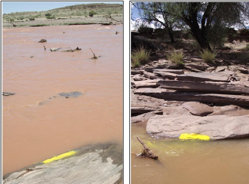
*Figure 7. Examples of stages marked on 16 February 2012 (for subsequent surveying during June 2012), corresponding to a discharge of 10 m<sup>3</sup>/s measured at the Seeheim gauge*
