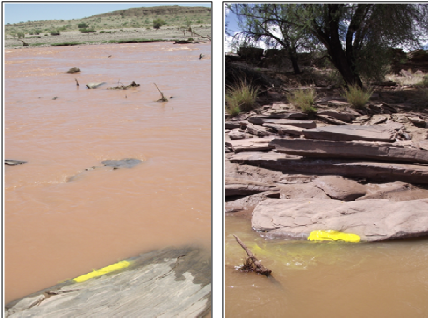
Figure 7. Examples of stages marked on 16 February 2012 (for subsequent surveying during June 2012), corresponding to a discharge of 10 m 3 /s measured at the Seeheim gauge
