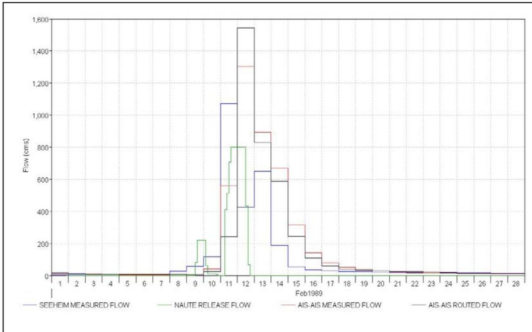
Figure C4. Discharge time-series plots of flows at the Seeheim gauge, and measured and routed flows (daily average) at the Ai-Ais gauge, for February 1989 (cms = m<sup>3</sup>/s)
