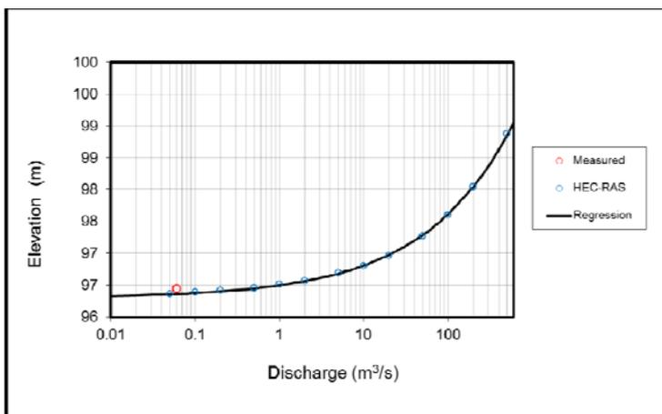
Figure B20. Stage-discharge relationships for cross-section 2.3 at EFR Fish 2 along the Fish River
