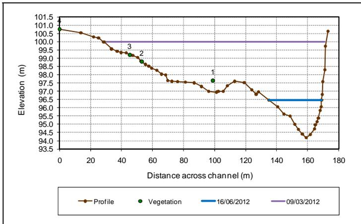
Figure B4. Cross-sectional profile 1.4 surveyed at EFR Fish 1 along the Fish River
