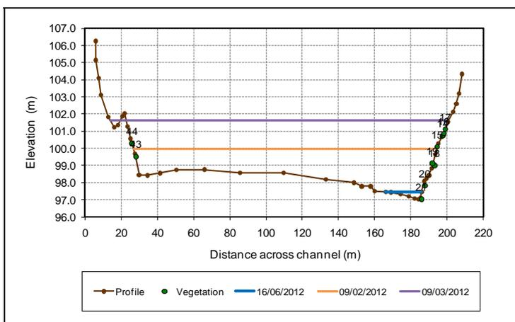
Figure B5. Cross-sectional profile 1.5 surveyed at EFR Fish 1 along the Fish River
