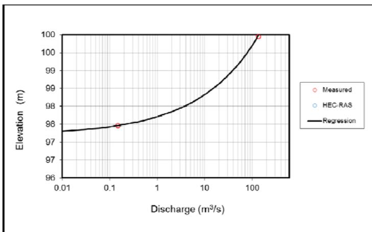
Figure B17. Stage-discharge relationships for cross-section 1.5 at EFR Fish 1 along the Fish River
