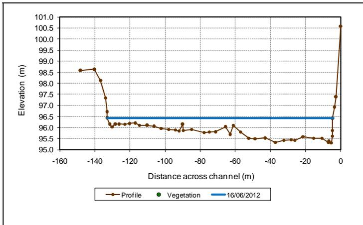
Figure B10. Cross-sectional profile 2.5 surveyed at EFR Fish 2 along the Fish River
