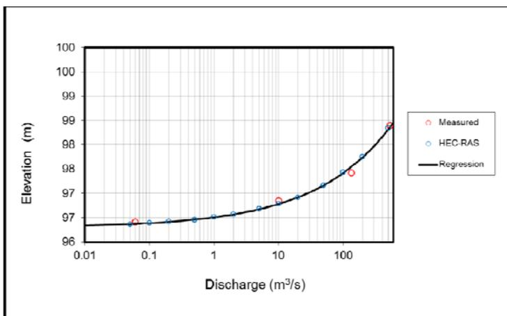
Figure B23. Stage-discharge relationships for cross-section 2.6 at EFR Fish 2 along the Fish River
