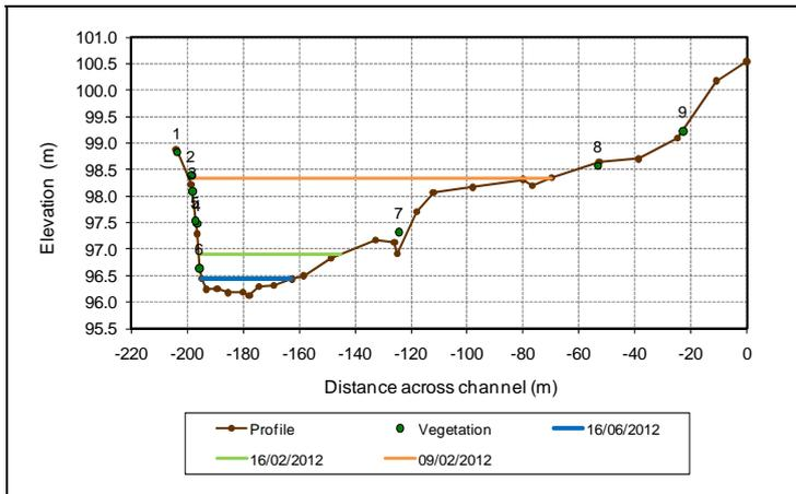
Figure B7. Cross-sectional profile 2.2 surveyed at EFR Fish 2 along the Fish River
