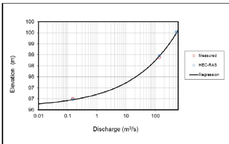
Figure B14. Stage-discharge relationships for cross-section 1.2 at EFR Fish 1 along the Fish River
