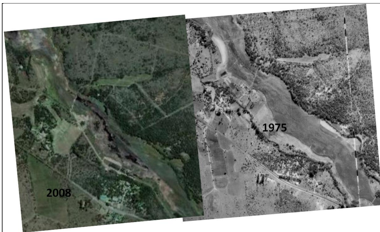
Figure E13 The road crossing has created an impoundment upstream. This has artificially increased the water level, and excavation in the wetland to create fishing and boating areas have created further disturbances in this area. Die off of the reeds has occurred between 1975 (right image) and 2008 (left image)
