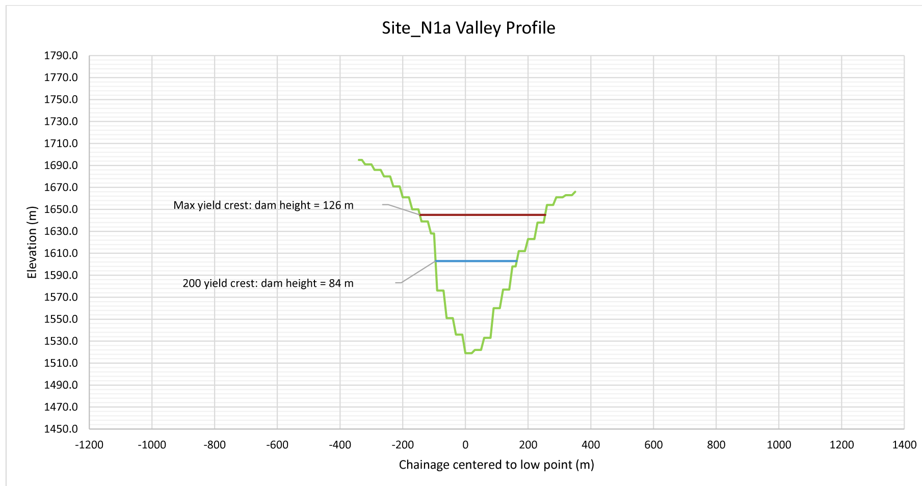
Figure 5: Dam valley profile with dam heights for a dam with 200 MCM/a yield and for a maximum a yield that equates to a capacity of 3 MAR
