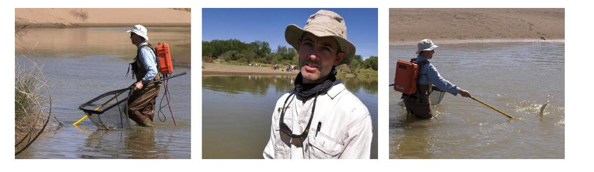
**Top:** Byron Grant is currently working on the fish using an electrofisher. The electrofishing apparatus deploys an electric field into the water, and the fish gets stunned by that. You're then able to net them without them swimming away.
