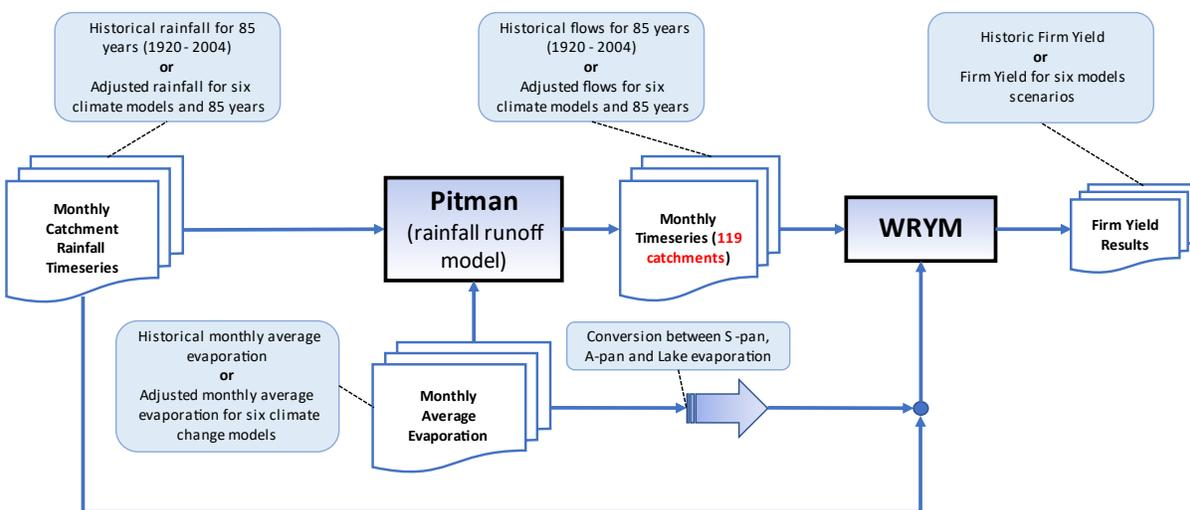
**Figure 2-1: Primary water resource modelling components & data flow**
