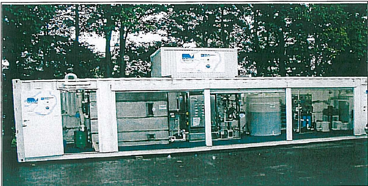
Figure 1: Portable WWTE in 12 metre shipping container used for 'sewer-mining', Melbourne, Australia. (Mallia, 2003).
