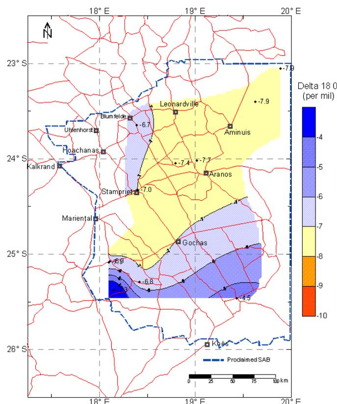
Figure 13: Oxygen-18 ratios ( $\delta^{18}\text{O}$ ) in the Nossob aquifer.
