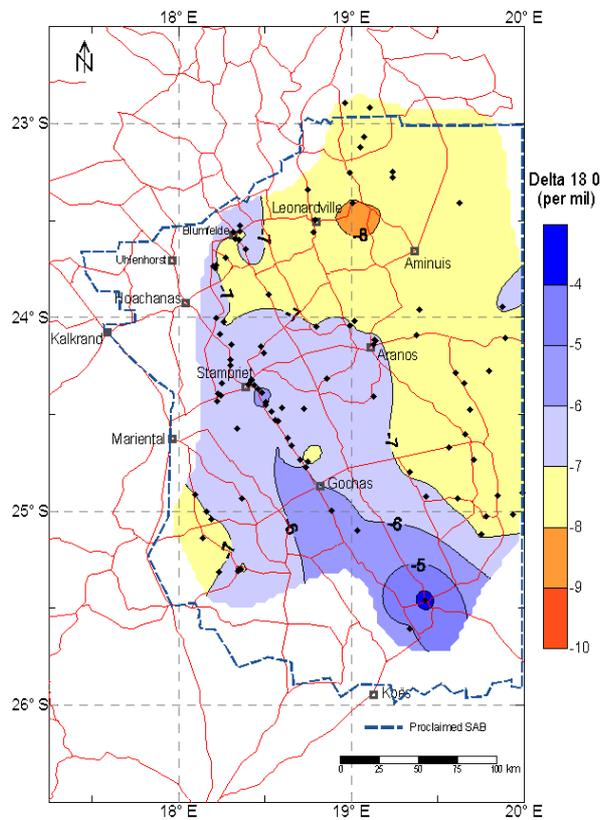
Figure 12: Oxygen-18 ratios ( $\delta^{18}\text{O}$ ) in the Auob aquifer.
