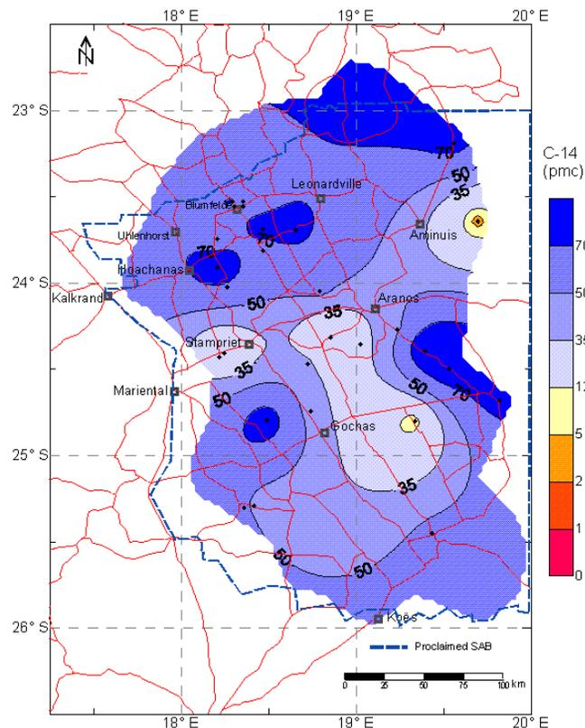
Figure 16a: Carbon-14 (pmc) in the unconfined aquifer system (Kalahari, basalt & Rietmond).
