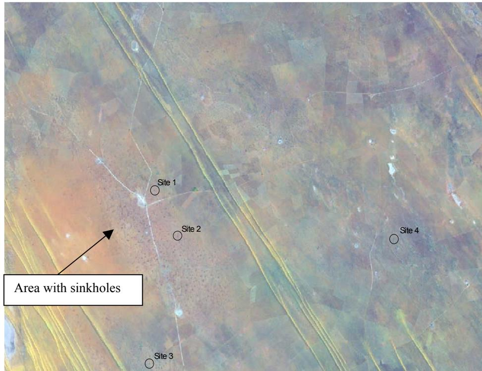
Figure 4: Dark dots near road intersection (Uhlenhorst) identified as potential sinkhole structures and approximate positions of the targeted drilling sites in the Uhlenhorst surrounding.
