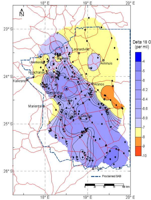
Figure 11: Oxygen-18 ratios ( $\delta^{18}\text{O}$ ) in the unconfined aquifers (Kalahari, basalt & Rietmond).
