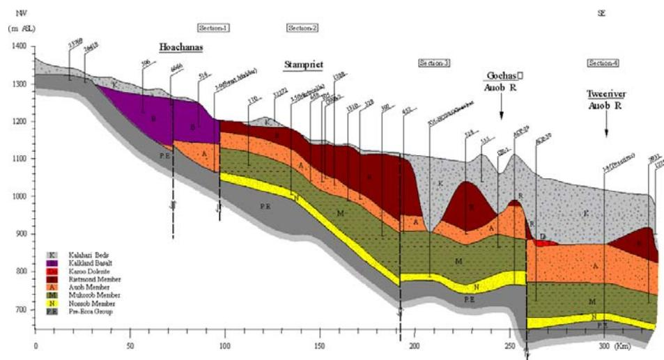
Figure 2: Cross-section through the SAB along the Auob River (after PCI, 2002).
