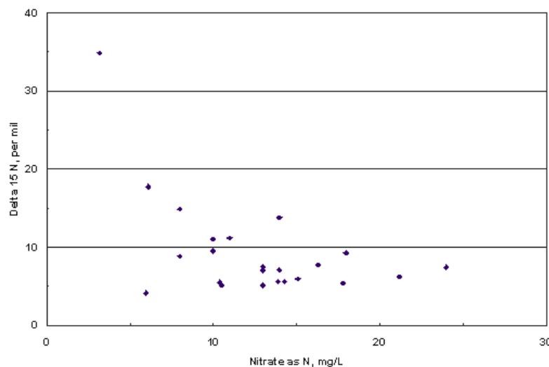
Figure 19:  $\delta^{15}\text{N}$  vs. Nitrate-N distribution in the Auob aquifer.
