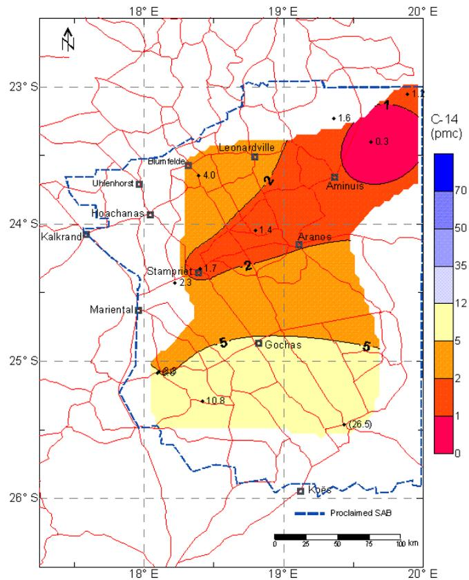
Figure 16d: Carbon-14 (pmc) in the Nossob aquifer.
