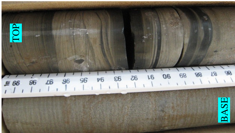
Figure 3.27 Upward-fining cycles within sandstones of facies association 2 in borehole ACP4. Clinorule scale in centimeters.
