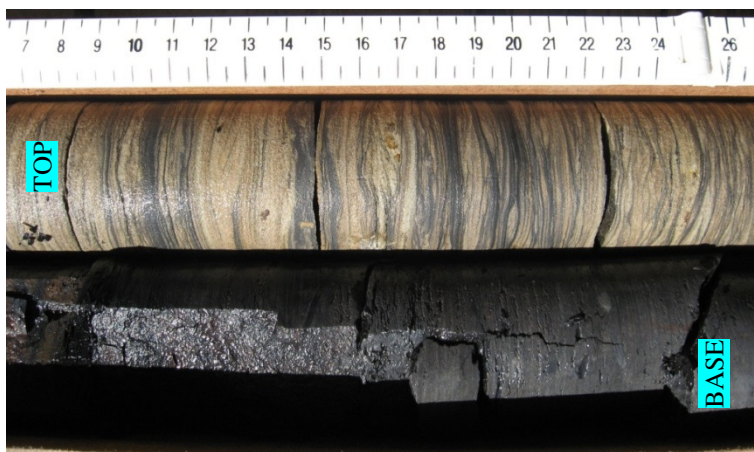
Figure 3.39 Carbonaceous mudrocks (Fc) with Planolites trace fossil grading upwards into ripple cross-laminated sandstones (Sr) of facies association 4, borehole ACP24. Clinorule scale in centimeters.
