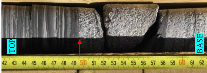
Figure 3.37 Poorly sorted, pebbly massive sandstones (Sm) with carbonaceous mudrock clast sharply overlain by laminated sandstone, siltstone and mudrock lithofacies (Fl). Borehole CKP8C. Tape measure scale in centimeters.
