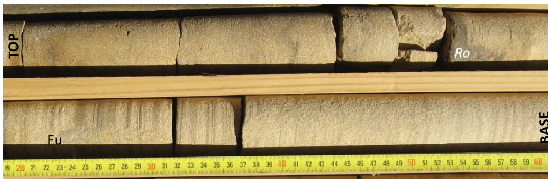
Figure 3.17 Massive sandstone (Sm) and horizontal laminated (Sh) sandstone with Rosselia (Ro) trace fossil and fugichnia (Fu), borehole W3. Tape measure scale in centimeters.
