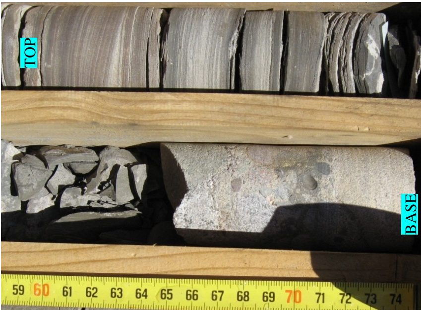
Figure 3.26 Clast-supported diamictite (Dcm) and alternating layers of sandstones and mudrocks displaying upward-fining cycles, borehole W3. Tape measure scale in centimeters.
