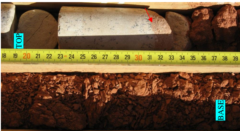
Figure 3.44 Reddish mudrocks of facies association 7 sharply overlain (erosive contact) by well sorted, fine-grained sandstones (Sm) of facies association 8 in borehole W1. Tape measure scale in centimeters.
