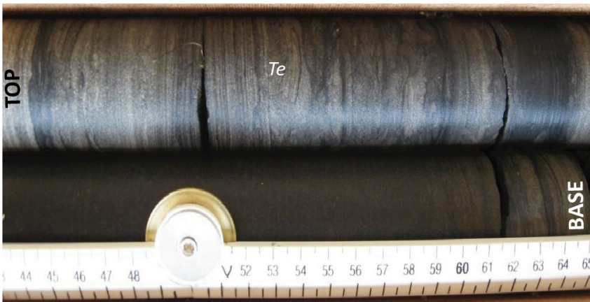
Figure 3.20 Laminated sandstone, siltstone and mudrock (Fl) with Teichichnus (Te) trace fossil, borehole ACP24. Clinorule scale in centimeters.
