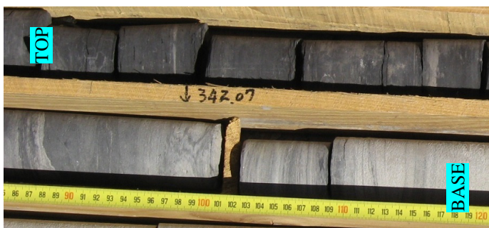
Figure 3.36 Upward-fining succession from sandstones (Sh, St, Sb) at the base grading upwards into bioturbated siltstone and mudrock (Fr) and carbonaceous mudrocks (Fc) interbedded with thin coals (C). Borehole CKP8C. Tape measure scale in centimeters.
