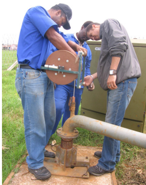
Measuring water levels in one of the boreholes considered for artificial recharge
