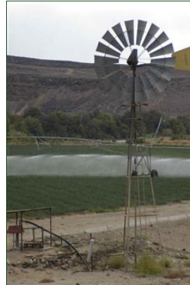
A wind-pump attached to a borehole in the Lower Orange River region. Source: Vogel 2009 ( click to enlarge )
