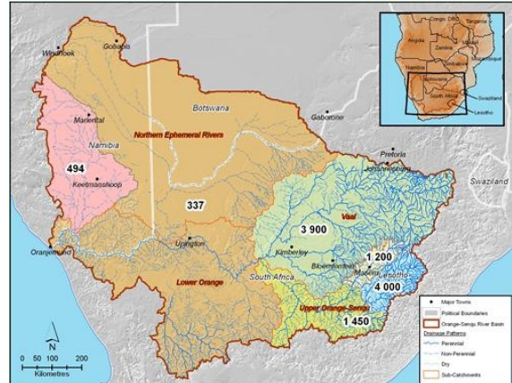
Approximate water balance for natural runoff in the Orange-Senqu River basin. Source: Hatfield 2009, after ORASECOM 2007f (click to enlarge)
