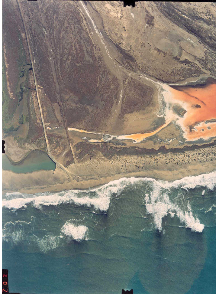
Figure 3 Approximately 90 % of the salt marsh in the present desertified area has been lost (Photo source: CSIR, November 1986). This was as a result of leakage of diamond-mining process plant water, the effect of windblown dried slimes dam sediment, construction of flood protection works and beach access road, and the elimination of tidal exchange into the wetland due to a dyke constructed at the river mouth.
