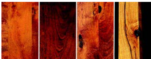
variation in boards stained knots filled cracks filled
