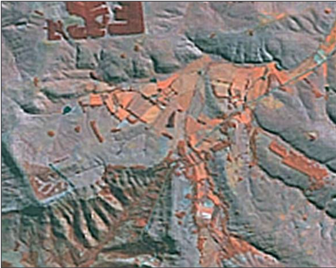
Figure 39. Crisp spatially enhanced (and run through cubic convolution model) Landsat ETM image
